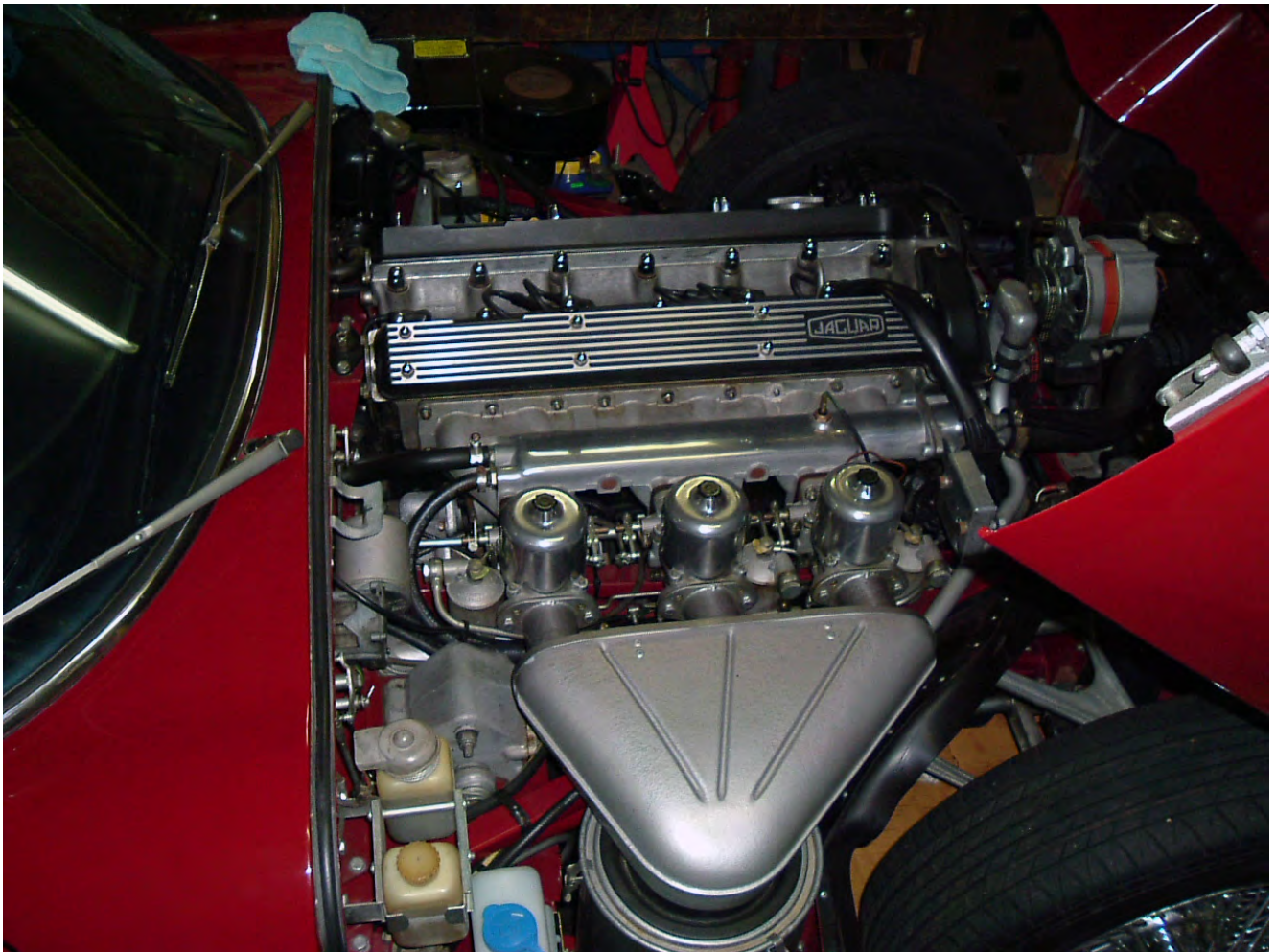
Cherry Ripe 2008 – Note the neat air conditioning vents and the high mounted alternator to allow for the positioning of the (original) air conditioner compressor (near side of engine)
